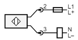
Note miniature fuse to IEC60127-2 sheet  $1 \le 2$  A fast acting
